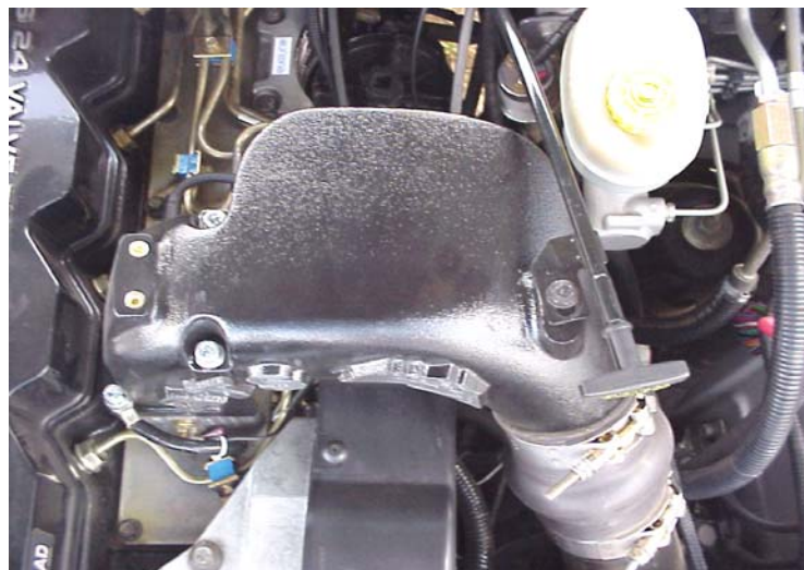
Figure 4 - Arc-Flow Intake Manifold After Installation
